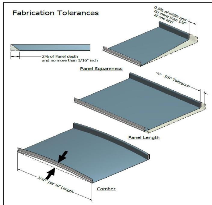
**Figure 2: MCA Fabrication Tolerances**
