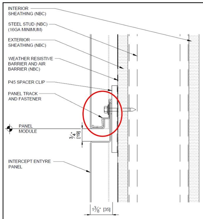
**Figure 1: Intercept Horizontal Panel Joint – Horizontal Application**
